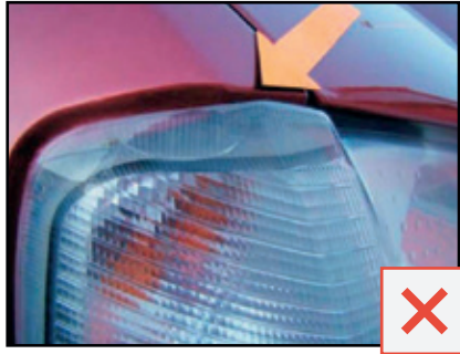
Cracks are not acceptable.
