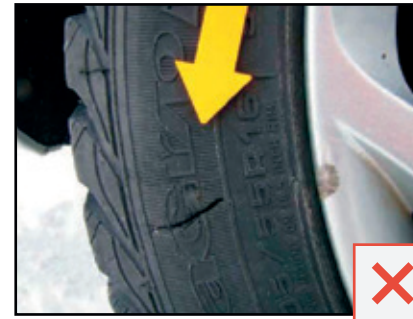
Damaged tyres are not acceptable.
