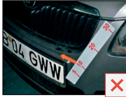
Peeling paint is not acceptable.
