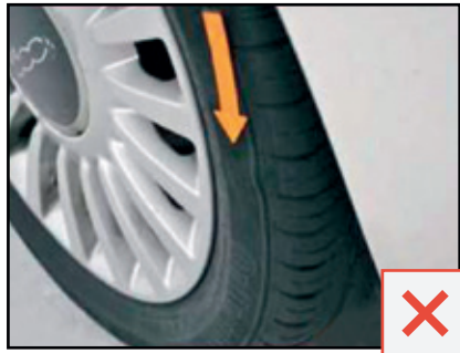
Tyres damages are not acceptable.
