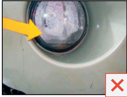
Damages of the fog lamps are not acceptable.
