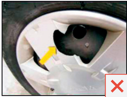
Wheel cover - broken is not acceptable.
